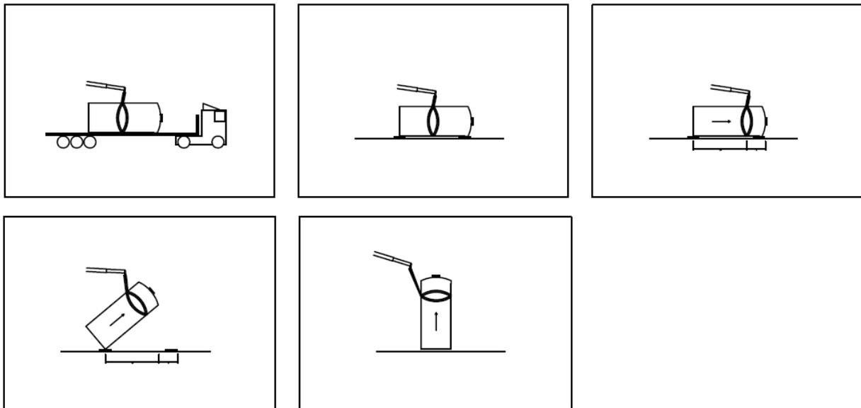
For large tanks is recommended to use two (2) cranes lacing tank from both sides with polyester slings. If will be lifted at once by both cranes avoiding any contact / impact against floor.
