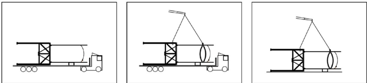
To put Silo in vertical position, it will be necessary two (2) mobile crane, one for each of slings fixed at the tank. Carefully lifting the tank, it will be placed in vertical position, avoiding dragging the tank or hitting it, which could damage it.
