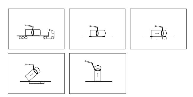
For large tanks is recommended to use two (2) cranes lacing tank from both sides with polyester slings. If will be lifted at once by both cranes avoiding any contact / impact against floor.
