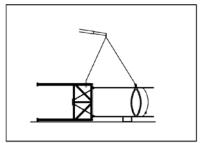
To put Silo in vertical position, it will be necessary two (2) mobile crane, one for each of slings fixed at the tank. Carefully lifting the tank, it will be placed in vertical position, avoiding dragging the tank or hitting it, which could damage it.
